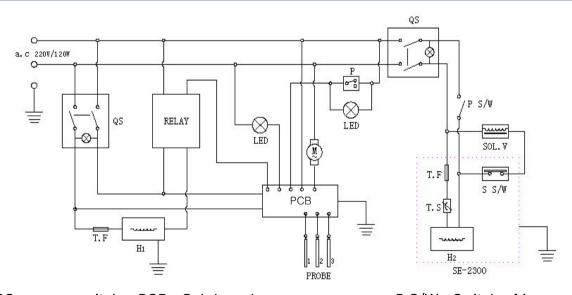
QS: power switch PCB: Pcb board
