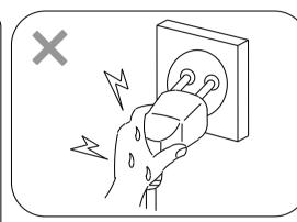
★ Wet hand is prohibited from pulling or inserting power plug
