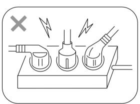
★ It must be used on the plug more than 120V/25A, 220V/15A individually.
