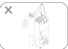
★ During product use, as baseplate temperature is very high, contact with any object should be avoided, Attention should be paid during use.
