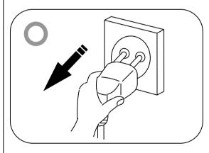
★ In case of pulling power plug, the hand must grasp the plug. Pulling plug in same method as pulling power wire with hand is prohibited.
