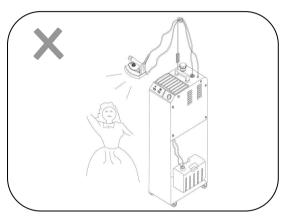
★ During product use, spraying at human body or contacting vapour is prohibited.
