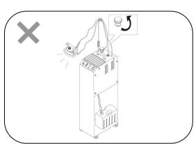
★During use of product, safety valve should not be contacted or opened.
